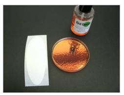
1. Apply the polymer and let dry. The polymer will stretch and not peel correctly if not fully cured.
