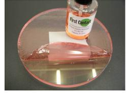
2. Allow to dry until there is no solvent smell, then carefully pull the mesh, once it starts to lift it will peel very easily.
